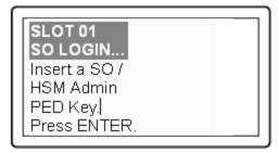
Authenticate as Security Officer by supplying the appropriate HSM SO PED Key that was imprinted during the HSM initialization step. The PED might prompt you for the numeric password PED PIN that might optionally have been assigned to the HSM SO PED Key. SafeNet PED provides the HSM SO authentication secret to the SafeNet HSM.
