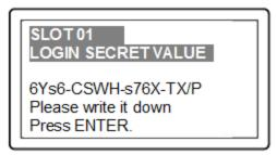
Record the Login Secret Value from the PED screen – write it down legibly – because it will never be shown again. This is the HSM Partition password, used to authenticate Client applications that wish to use the HSM Partition on the SafeNet Network HSM.
